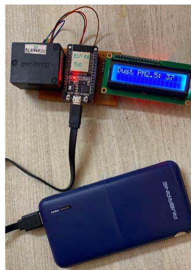
Latest iteration of the one AQM designed to engage viewers - All components are visible to indicate the simplicity and to focus on the Dust Sensor, and speak about its accuracy
