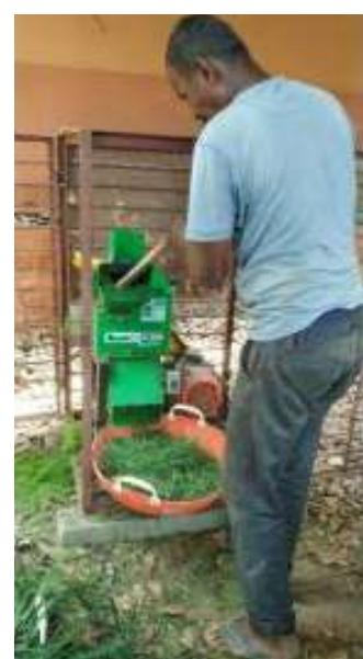
Feeding and pushing into shredder
